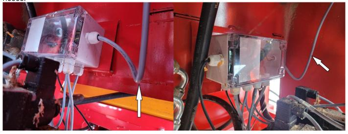
4. For machines with the box on top of them, it is not necessary to change the cable routing.
